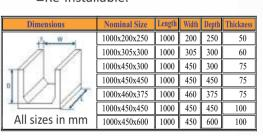
Precast Concrete U drains allow for speedier construction of Drains with minimum site work. We manufacture a full range of U shaped drains. These drains come in different Sizes and can be customised as per your needs.
